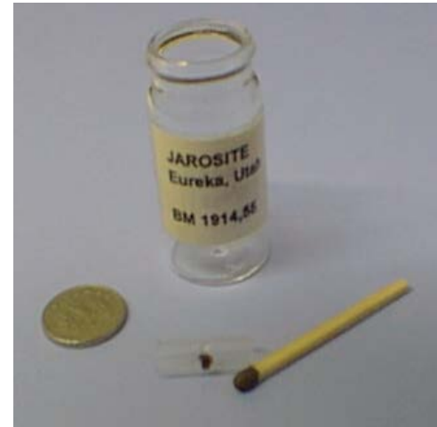
natural sample of \text{KFe}_3(\text{SO}_4)_2(\text{OH})_6 4mm 3 ; 15mg
